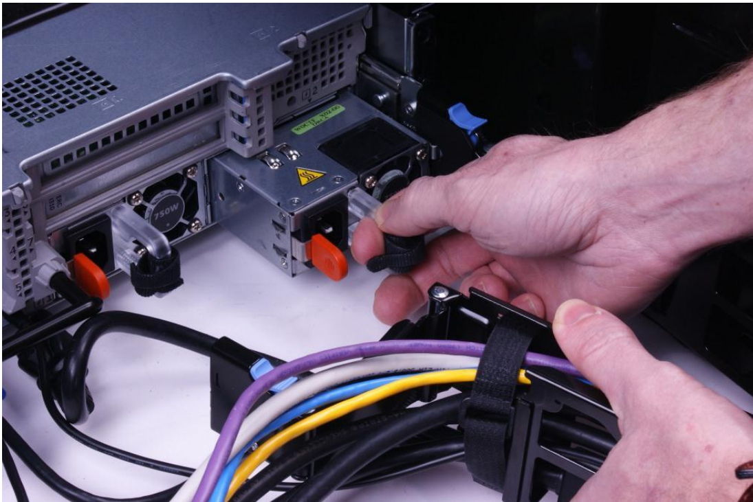
Figure 8. Replacing the outer power supply
